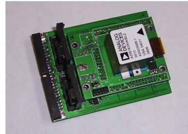
Fig. 17. Custom-designed auto-pilot system for robotic fish.
